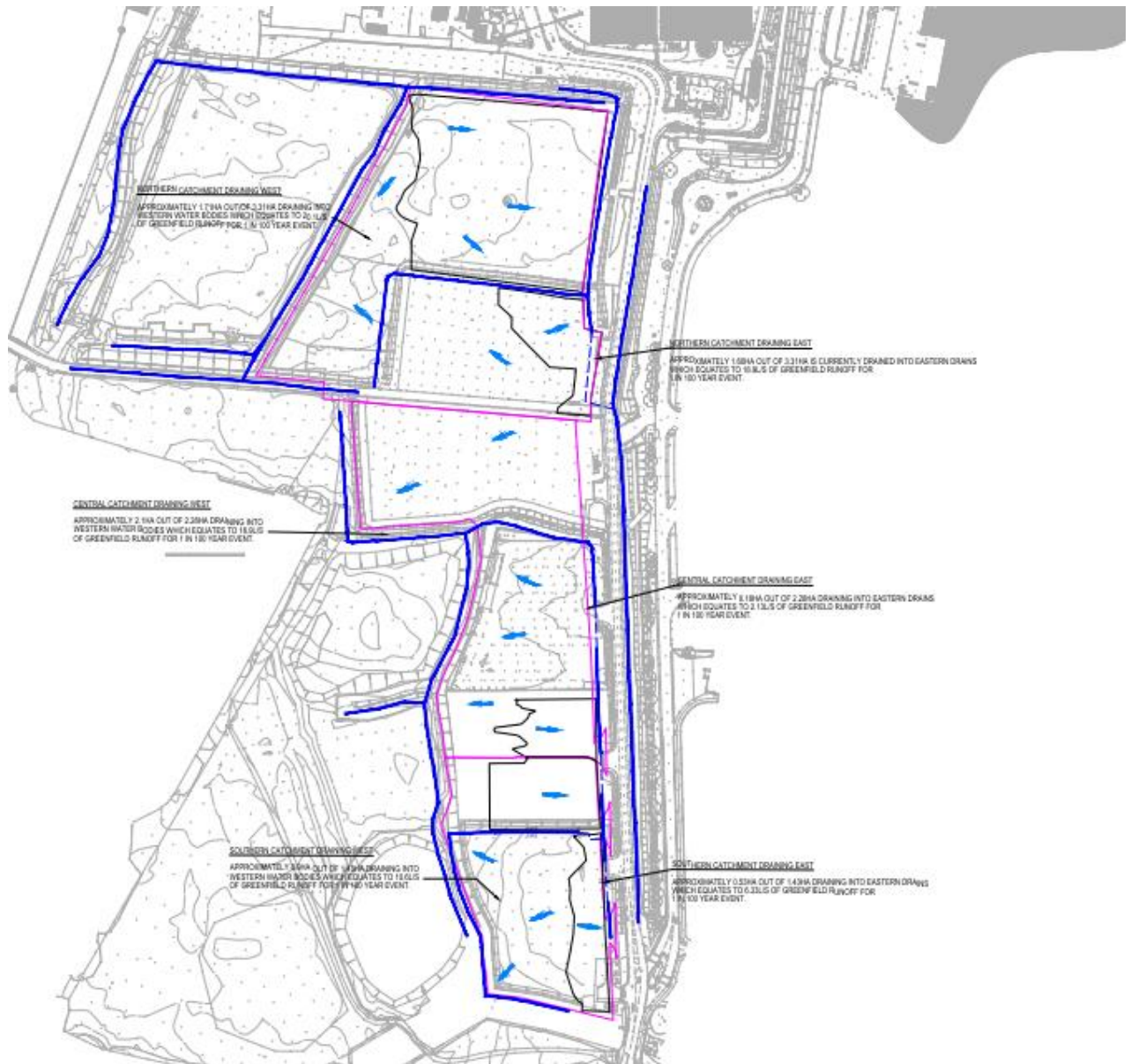
Figure 2-2: Existing Drainage Catchment
